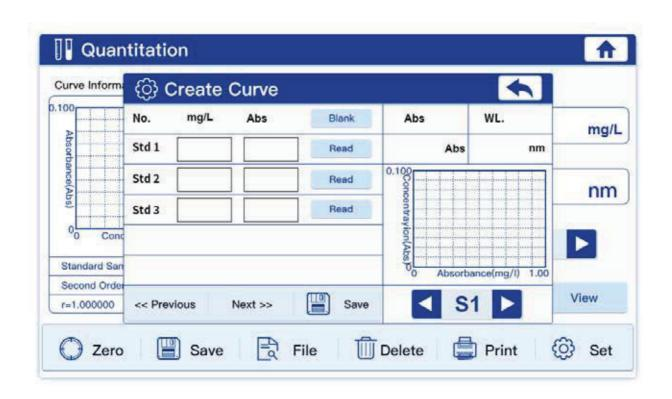
Press Save in the small window to continue, if necessary, please calibrate absorbance by pressing Blank button.
