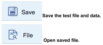
After you do some test, first press save button, then open files. Otherwise, the system will remind you Data Modified, Save Record? You can press OK to save test records or cancel it to continue open other files.
