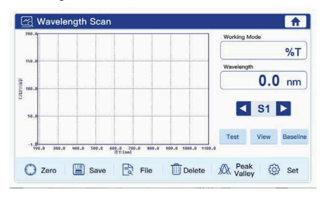
In the set wavelength range with a certain wavelength interval to record the absorbance, transmittance or energy value of the sample which will be plotted in the map and can be seen in the sample absorbance, transmittance, and the energy value trends at different wavelengths.
