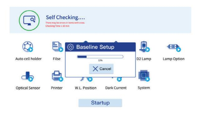
After you create the system baseline or cancel it, the machine will start preheat automatically and last twenty minutes. We suggest you finishing preheat process, otherwise it may influence the instrument's accuracy and stability.
