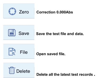
This function cannot be used to delete saved files.
