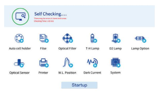
**[Files]**: to check instrument's built-in Flash file system if they are damaged or not. If there is an error, please format file system.
