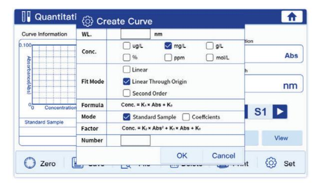
You can input wavelength, highlight concentration units and fit modes (linear, linear through origin and polynomial 2nd order), test mode (standard samples or coefficients). When you use coefficients mode, it will show the relevant factors in the factor column. If you highlight standard sample mode, you need to input the number of standard samples (at least two).
