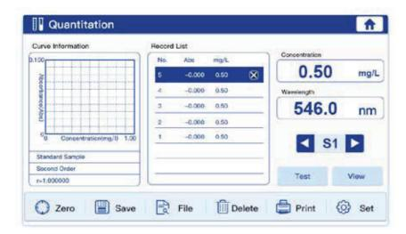
After that, you can do the test, view test results, save and open files, delete test records, print and set the concentration units.
