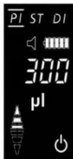
② If the pipetting volume is set less than 30% of the total volume range of iPette+, and more than its minimum volume range, 50% of the set volume will be mixed.
