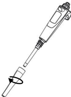
② Remove the ejector spring. Unscrew the piston cover anticlockwise and remove it.
