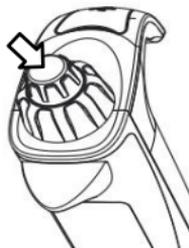
Pressing the **Parameter Knob** again after dispensing the final step liquid had been dispensing that use to drain the liquid which left in the Tip possible. the pipette will return to the aspiration conditions.
