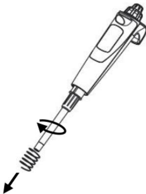
③ Separate the seal gasket and O ring from piston cover.
