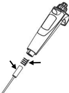
⑤ Clean the above-mentioned parts with 75% ethanol, or sterilize the parts at 121°C, 1 bar overpressure for 20 minutes.
