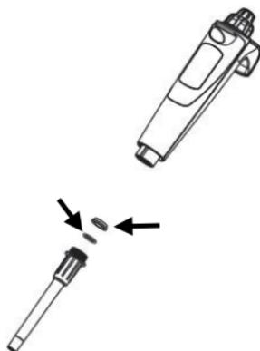
④ Separate the remaining piston from piston spring.
