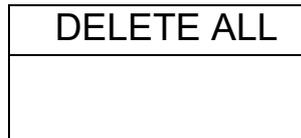
When the selection shows DELETE ALL, press **[Setup/Enter]** to delete all test results. The display will ask if you are sure you want to delete all results. Press **[Setup/Enter]** again. The display will count down from 99 to 0 during the time it takes to remove all the files.
