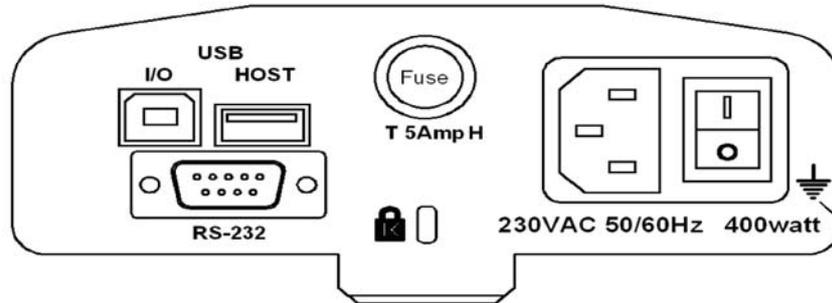
The rear panel has connectors for the data interface, fuse holder, security lock location and power supply input.
