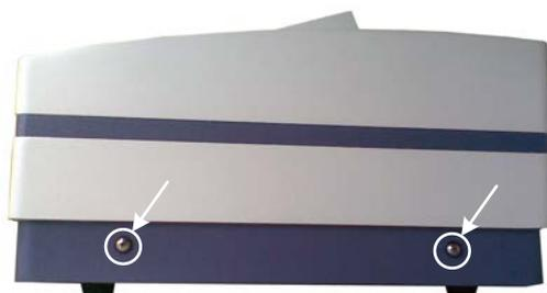
**Step 4. Open the cover of the light chamber**
