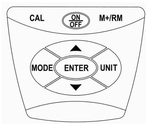
Keypad operations: Short press— <1.5 seconds; Long press — >2seconds.
