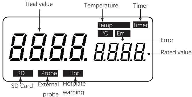
Figure 5 LCD digital model
