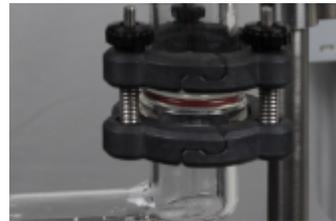
Screw-lock connection for excellent condenser sealing, and easy installation
