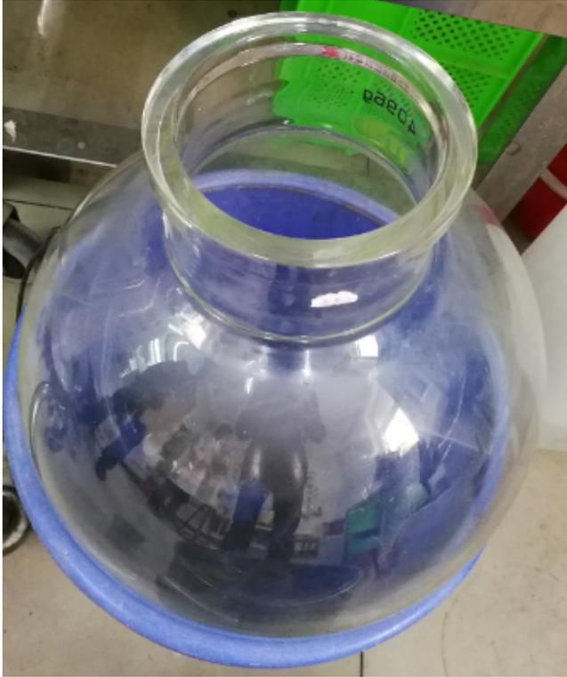
Wide-mouth sample flask, for faster filling and easier cleaning
