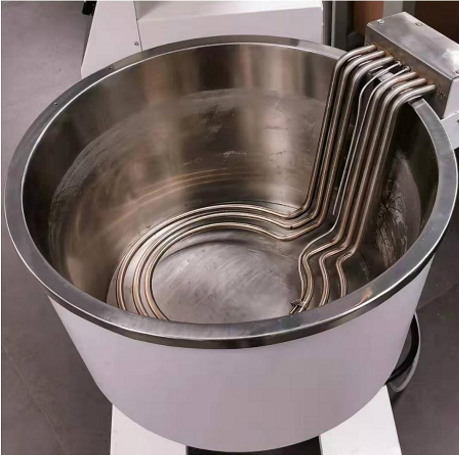
Heating bath with external heating coil provides higher heating efficiency, and easy maintenance.
