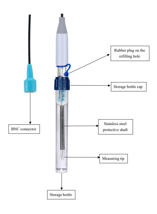
LabSen<sup>®</sup> pH electrodes are made with proprietary sensor technologies and key components from Switzerland. LabSen<sup>®</sup> 241-3 Micro pH electrode is designed for high-accuracy pH measurement of microvolume samples in small containers such as test tubes, microplates, and centrifuge tubes.
