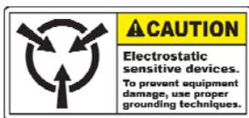
Avoid operating in high static areas, or weighing high static materials, such as plastics or powders, as this may damage electronics and affect measurements. Use grounding mats or bonding straps to reduce potential
