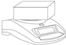
Keep the balance clean. Do not stack material on the balance / balance pan when it is not in use. The Highland has a stacking feature for stacking more than one unit on top of each other which does not apply weight to the pan. For more details on this see the section on storing.
