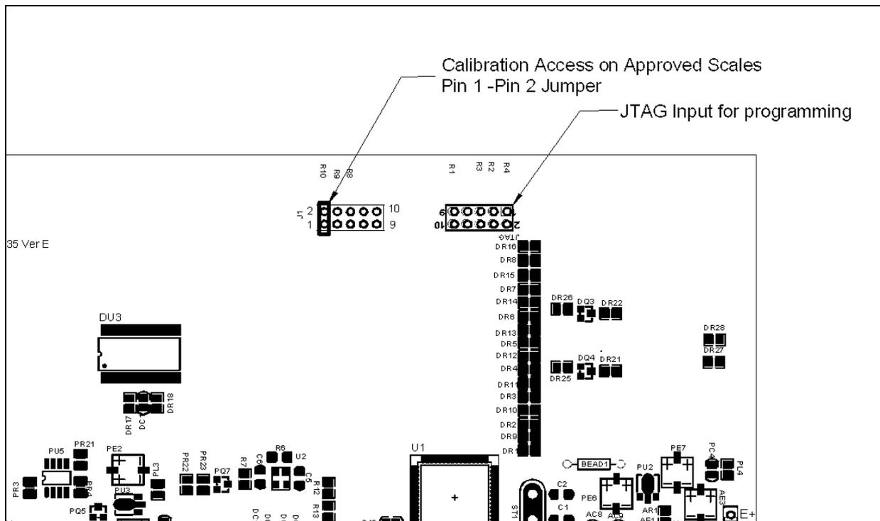
Apply power to the indicator. If the jumper has been used the display will ask for a code number, **"Pn "** on the Weight Display immediately. Or press the [Tare] key during the time the calibration counters are being displayed.
