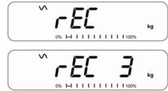
**NOTE:** If the recalled limit is for parts counting or percent weighing, the display will show the last sample value used, ready for a new sample to be counted.
