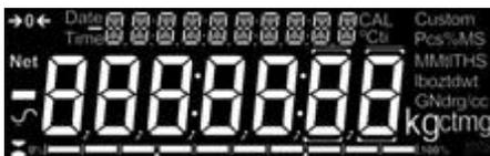
Once a suitable warm-up period is complete and you are ready to start weighing, place an item to be weighed on the balance. A stable symbol  $\curvearrowright$  is shown when the balance is in stable condition. It will turn off if the balance is not stable.
