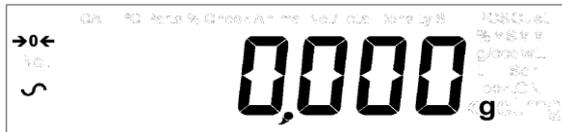
The display will show zero reading along with the zero symbol "→0←" and the weighing unit last used. If automatic time calibration is enabled the balance will calibrate 15 minutes after power up, or again after the pre-set time interval.
