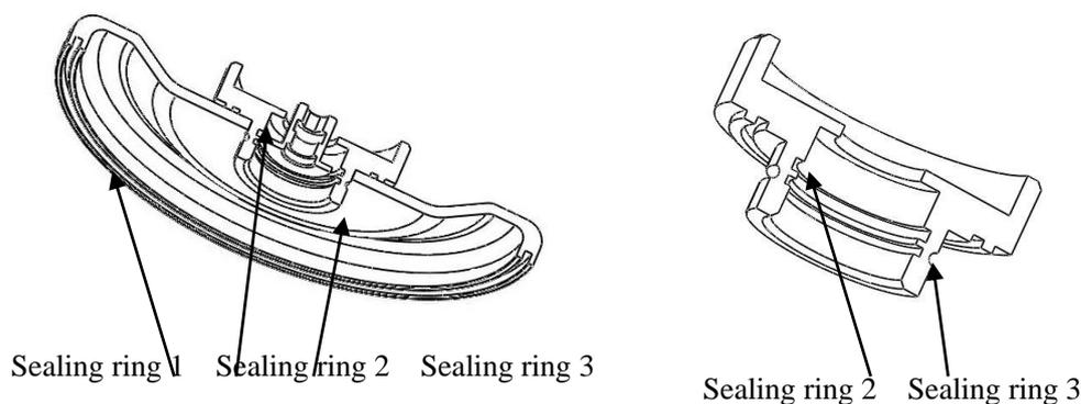
Fig. 9-1 Rotor sealing ring
