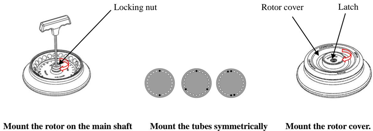
Fig. 8-4. Rotor installation
