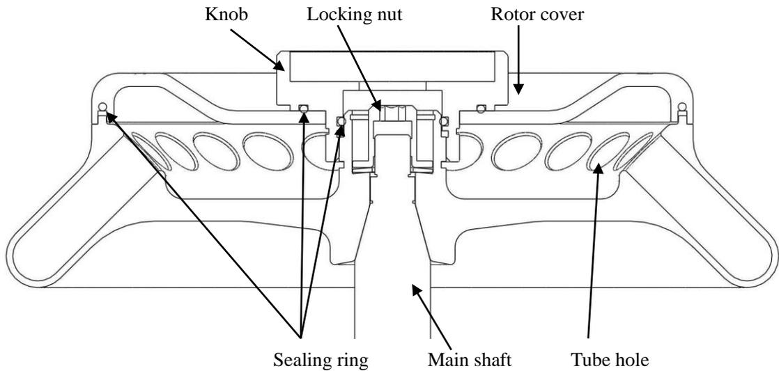
Fig. 11-1 Rotor structure
