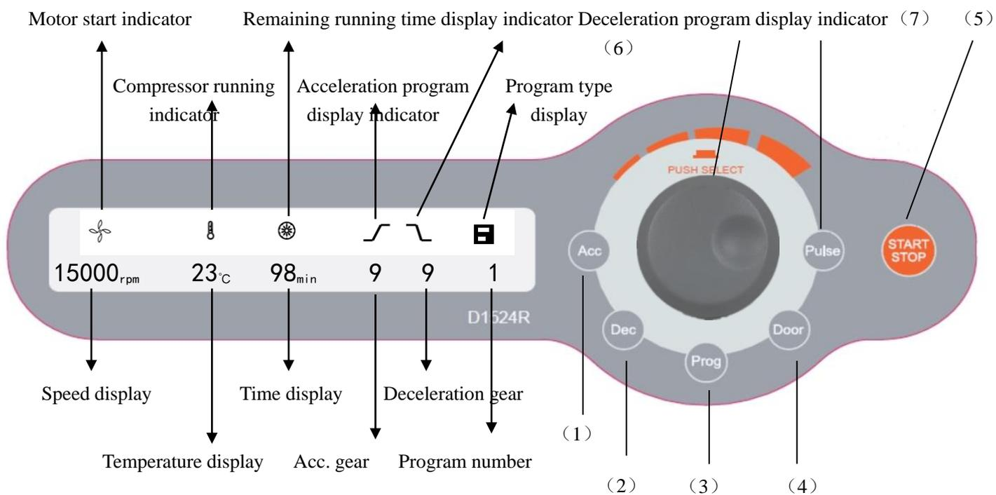
Fig. 6.1 Schematics of operating panel
