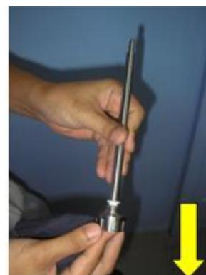
remove rotor, stator and teflon bearing
