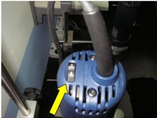
The speed is selected by the control knob on the top of the drive. Approximate rpm of the drive is:
