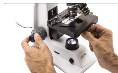
Regulation of diaphragm aperture
