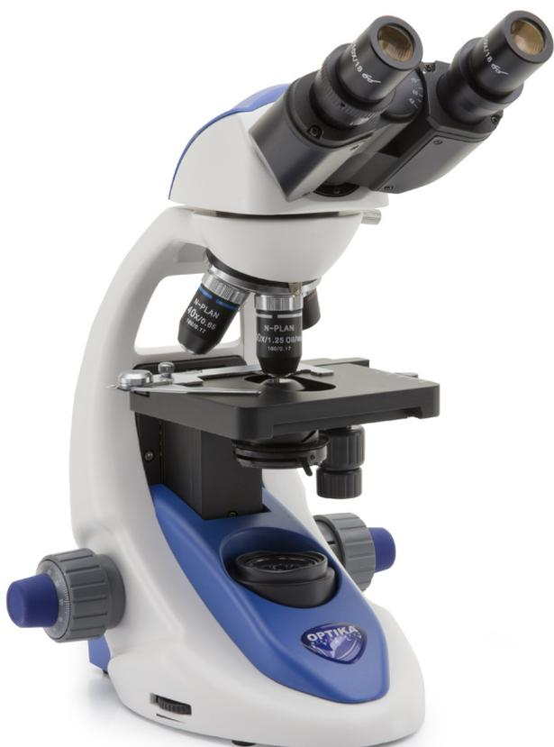
Binocular microscope ideal for teachers and secondary schools, with four N-PLAN objectives (1000x), FN 18 high eyepoint, finite optical system, coaxial focusing, mechanical stage, Abbe condenser and powerful, uniform, white color temperature 3 W **X-LED<sup>2</sup>** illumination. Slim and easy to carry, yet sturdy and resistant, it is equipped with all the main controls to start learning how to use an advanced microscope and with long lasting LED illumination to provide over 20 years of use
