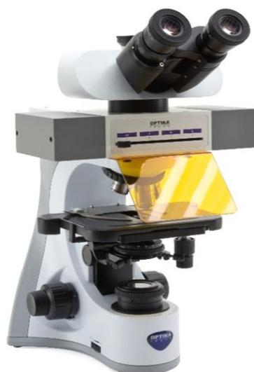
*Trinocular LED fluorescence microscope,
