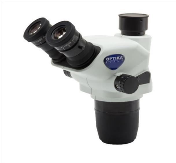
*Trinocular stereozoom microscope head,
