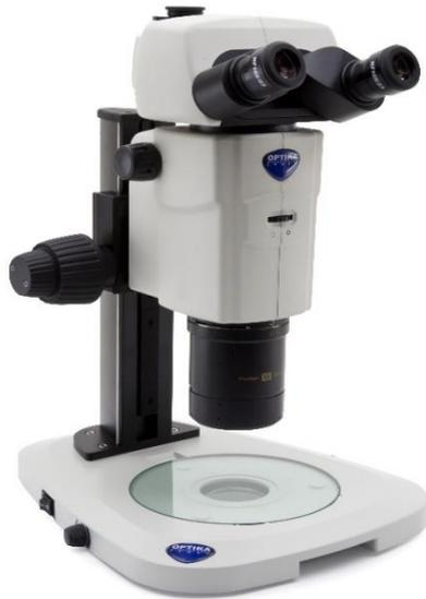
*CMO stereomicroscope, 7.5x-135x, Zoom ratio 18:1, multi-plug*
