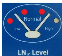
The  $LN_2$  level gauge on the face of the control indicates level by lighting the appropriate LED if a thermistor is submerged in  $LN_2$ . In the picture, the Low Alarm thermistor, the Start Fill thermistor and the Stop Fill Thermistor are all submerged in  $LN_2$ .
